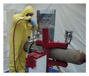
Weathering can remove all markings on a gas cylinder. A special tent must be used and filled with nitrogen gas to avoid explosions in order to safely test and remove the contents.
