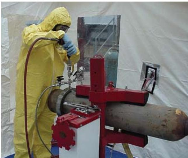
**Weathering can remove all markings on a gas cylinder. A special tent must be used and filled with nitrogen gas to avoid explosions in order to safely test and remove the contents.**
