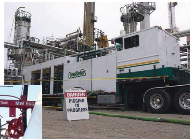
Clean Harbors' closed loop pigging process uses a high-volume, low-pressure water pumping system to propel its patented bi-directional pigs through pipes and coils to effect cleaning.
