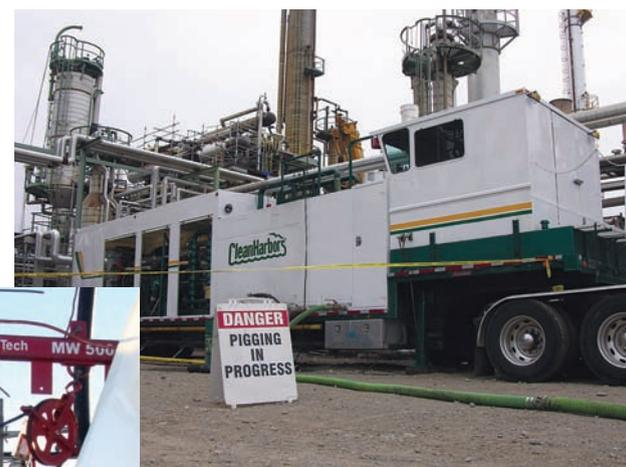
Clean Harbors' closed loop pigging process uses a high-volume, low-pressure water pumping system to propel its patented bi-directional pigs through pipes and coils to effect cleaning.
