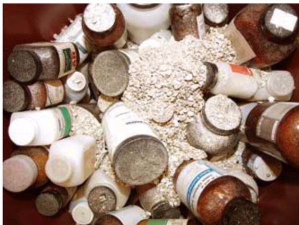
*<< An example of poor packaging of laboratory chemicals for disposal. Poor packaging can cause breakage. If the materials were not properly categorized and segregated, materials can potentially react.*
