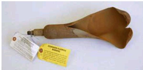
**<< Laboratory lecture bottle once contained hydrogen fluoride. When stored over two years, hydrogen fluoride reacts with the iron in the bottle and begins to form hydrogen gas. The hydrogen gas builds up over time to the point where the bottle can rupture.**
